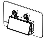
**2** Fix four screws on the installation surface.
