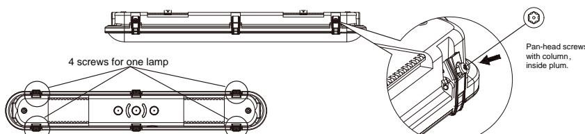
Close the lamp housing by snapping the side clamps into place. Then, insert and tighten the pan-headed fastening screws to securely lock the lamp (Allen key is available as accessory for separate purchase).
