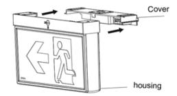
3. Knock out the cable entry in the middle at back and connect to the mains
