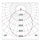
Unit: cd – C0/180 106.2deg – C90/270 106.2deg Photometric diagram shown is for 4000K output.
