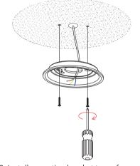
3. Install mounting bracket to surface.
