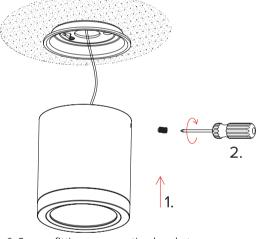
Secure fitting on mounting bracket using screws supplied.
