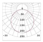
Unit: cd – C0/180 114.5deg – C90/270 114.5deg Photometric diagram shown is for 4000K output.
