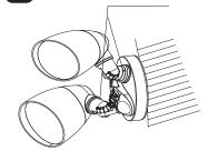
2 Pull the main through gasket and wiring base
