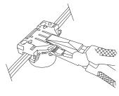
3. Tightly squeeze the cover with pliers as shown until both clips latch.
