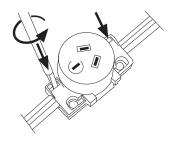
4. If required, re-open by inserting flat blade screwdriver and twist to release both clips.
