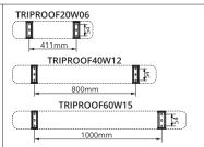
2. Measure hole positions on mounting surface. Fasten brackets to mounting surface.
