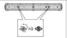
5. Unlock and remove gear tray.
