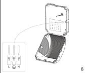
Terminate cables into terminal block ensuring correct polarity and the luminaire is earthed.
