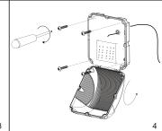
Open fitting via captive screws around edge of luminaire.
