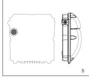
Side entry cabling to be sealed and fixed with appropriately IP rated M20 Cable glands.
