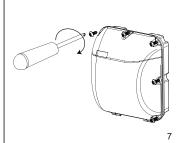
Close fitting via captive screws around edge of luminaire.
