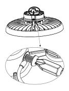
**STEP 4:** If required, adjust the bracket angle to suit.
