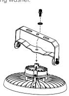
**STEP 3:** Secure the wiring harness onto the mounting bracket.
