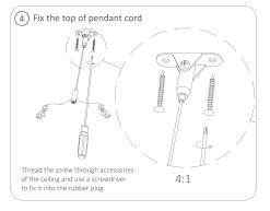
4. Thread the screws through accessory holes into the ceiling and use a screwdriver to fix it into the rubber plugs.
