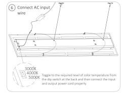
6. Connect AC input wire, toggle the dip switch at the back of the luminaire to the required colour temperature setting, and then connect the input and output power cord properly.
