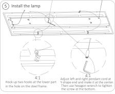
5. Install the luminaire: hook up two hooks at the lower part in the hole on the steel frame. Adjust left and right pendant cord at Y-shape end to make centred. Then use hexagon wrench to tighten the screw at the bottom.
