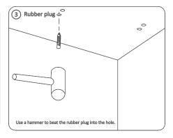
3. Using a hammer, beat the four rubber plugs into the four holes.
