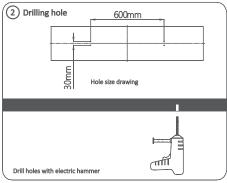
2. Drill four holes as specified in the illustration.
