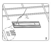
2. Toggle the dip switch at the back of the luminaire to the required colour temperature setting, and then connect the input and output power cord properly.
