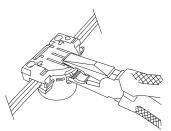
3. Tightly squeeze the cover with pliers as shown until both clips latch.
