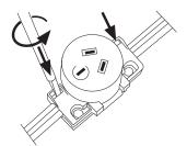
If required, re-open by inserting flat blade screwdriver and twist to release both clips. Note: To ensure adequate connection, do not reinstall in the same position on the cable.
